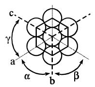
Note: There are three unit cells shown. In each unit cell, there are parts of eight atoms at the corners of each unit cell. For the atoms at the 30° corners only 1/12 of the atoms are in the cell while 1/6 of each atom at the 60° angles are in the cell. Therefore there are a total of 2 atoms in each cell.
